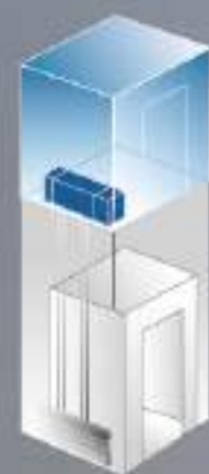
Small machine room
